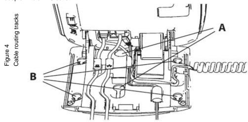
**Step 8: Wall-mount your phone (optional).** Your IPPhone1140E can be mounted either by: (Method A) using the mounting holes on the bottom of the phone stand, or (Method B) using a traditional style wall-mount box with RJ-45 connector and 15-cm (6-inch) CAT5e cable (not provided).
